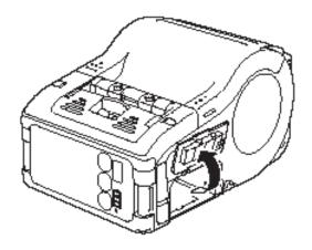
3. Push aside the gray latch (1) in the compartment, grasp the tab (2) on the top of the battery pack (3) and pull it out.
